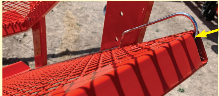
Clean-out rod to clean out soil/debris from throat and shoes.
