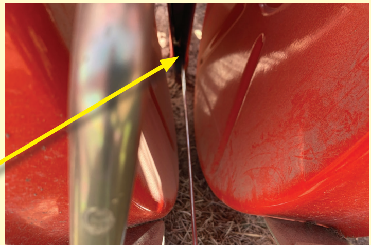
Clean-out rod to clean out soil/debris from throat and shoes.
